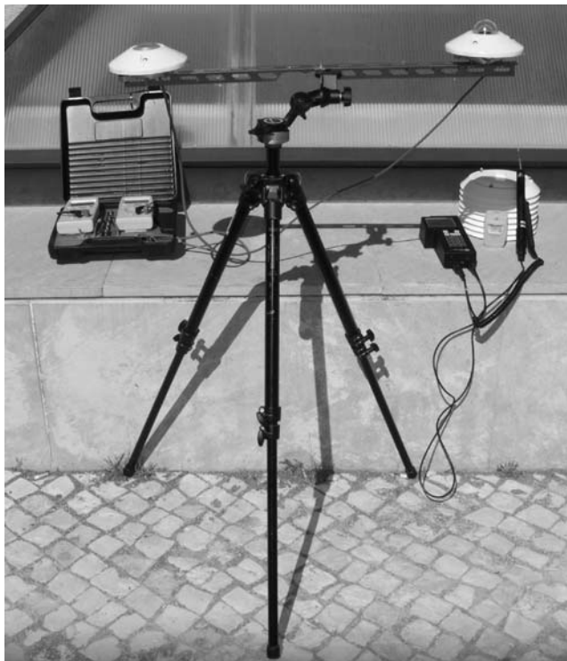
Fig. 3 Equipment used to measure weather parameters. Foreground: right pyranometer, left pyrgeometer. Background: right Testo data logger with its temperature, relative humidity and wind speed measuring probes, with the Tinytag thermohygrometer with its shelter behind
